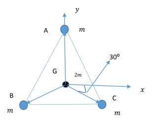
Three equal masses are placed at the three vertices of the triangle ABC. A mass 2m is placed at the centroid G.
