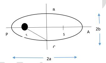
An ellipse traced out by a planet around the sun. The closest point is P and the farthest point is A, P is called the perihelion and A the aphelion. The semimajor axis is half the distance AP.
